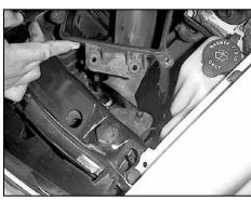
8. Pull the air box upward firmly to release the grommets from the retainer bracket.
