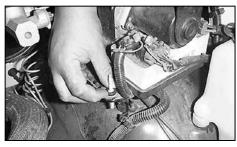
20. Install the 5/8" OD grommet and a flat washer over the original air box mounting stud.
