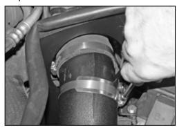
39. Attach the saddle/bracket assembly to the secondary intake tube using the provided hose
