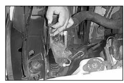
9. Pull the release tab and slide the retainer bracket upward to remove it from the radiator core support.
