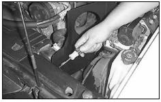
22. Install the heat shield and secure it with a provided self tapping screw.
