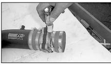
31. Install the second silicone step hose onto the exposed end of the mass air sensor and secure with the hose clamp provided.
