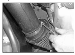
40. Install the air filter element onto the intake tube rotate, for best clearance and secure it with the provided hose clamp.
