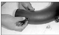
27. Install the 1" OD grommet into the hole in the primary intake tube.
